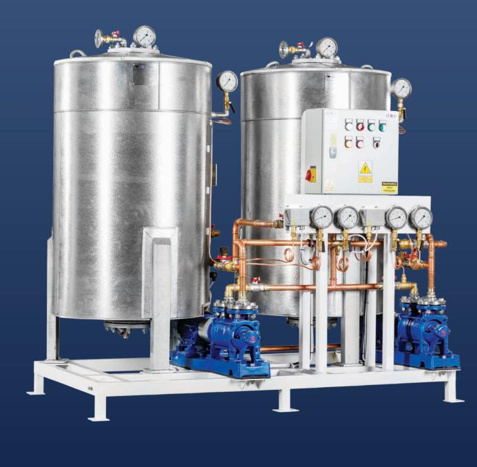
TANK TYPE: VERTICAL, DIAPHRAGM TYPE TANK CAPACITY: 400 L TANK MATERIAL: BLACK STEEL, HOT GALVANIZED TANK CERTIFICATE: LRS WORKING PRESSURE: 6 BAR MINERAL WOOL 20mm INSULATION 2x SELF-PRIMING PUMPS 2,5 m3/h / 6 BAR PUMP TYPE SELF PRIMING (SIDE CHANELL TYPE)
