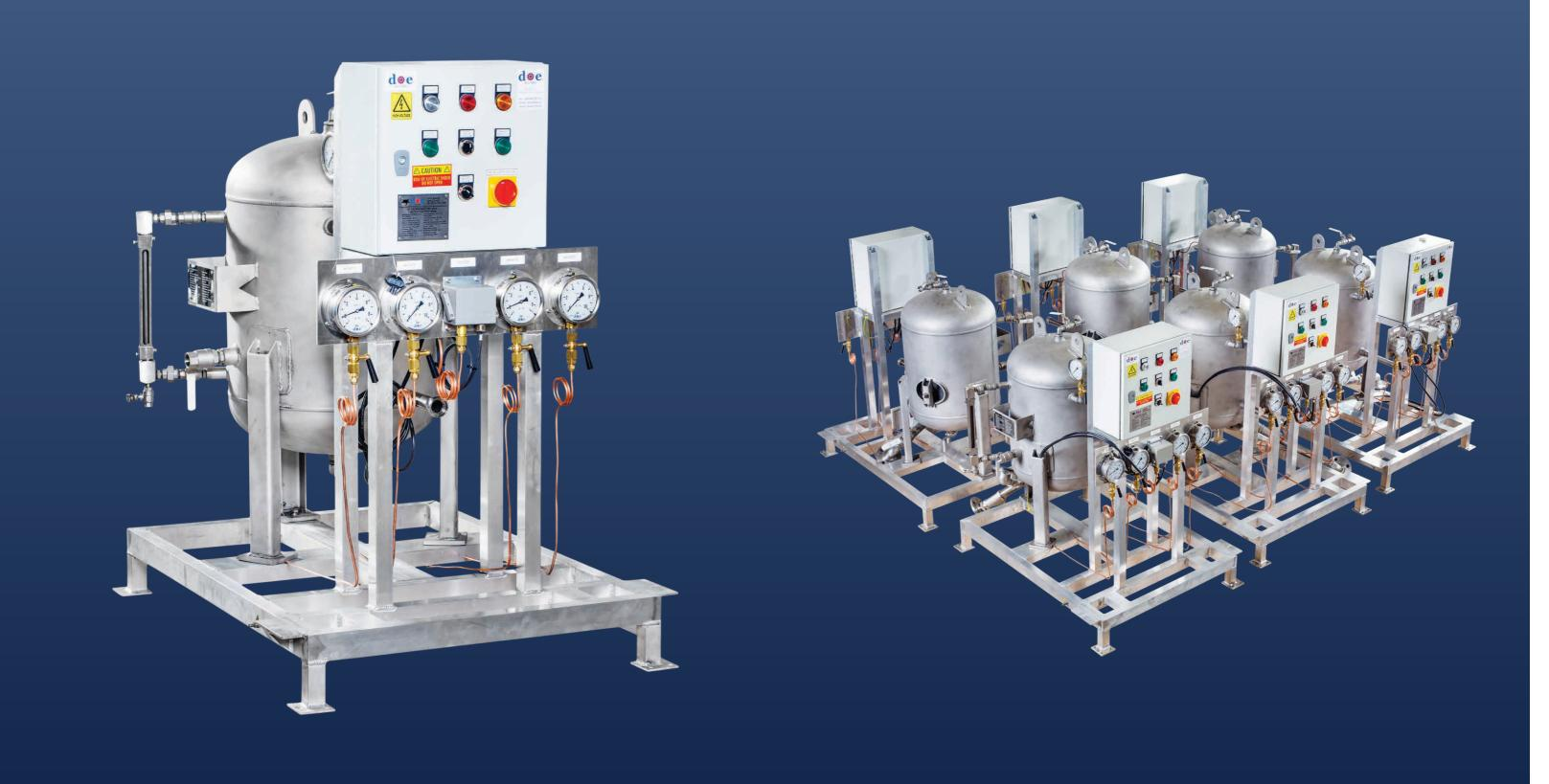
6X HYDROPHORE SYSTEM 100L, EQUIPPED WITH: TURTLE 100L STAINLESS STEAL (SS 321) COMPLETE PIPING COMMON SKID WORKING PRESSURE 4BAR POWER INSTALLED 3KW
