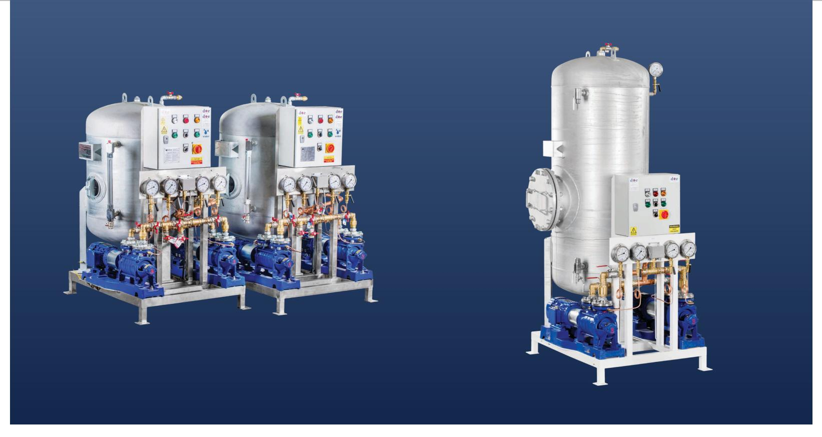
TYPE: VERTICAL, CYLINDRICAL CAPACITY: 300 LITRES MATERIAL: BLACK STEEL, GALVANIZED COMMON FRAME (SKID) MADE OF STAINLESS STEEL TYPE: AISI 304 SELF-PRIMING PUMP, 3 m3/h, 5 BAR – 2 PCS. TYPE: VERTICAL, CYLINDRICAL CAPACITY: 600 LITRES MATERIAL: GALVANIZED BLACK STEEL WORKING PRESSURE: 5 BAR COMMON FRAME (SKID) – 1 PC ELECTRICAL BOX (CONTROL CABINET) FULLY EQUIPPED PROTECTION: IP55 04 SELF-PRIMING PUMP TYPE 4.5 m3/h, 4 bar – 2 PCS
